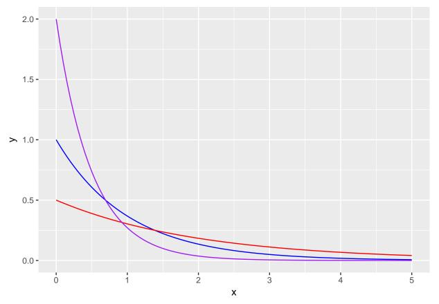
Example: Lifetime of a bulb is expected to be 10,000 hours, estimated with exponential distribution. What is the probability that the bulb will fail in the first 3,000 hours?
